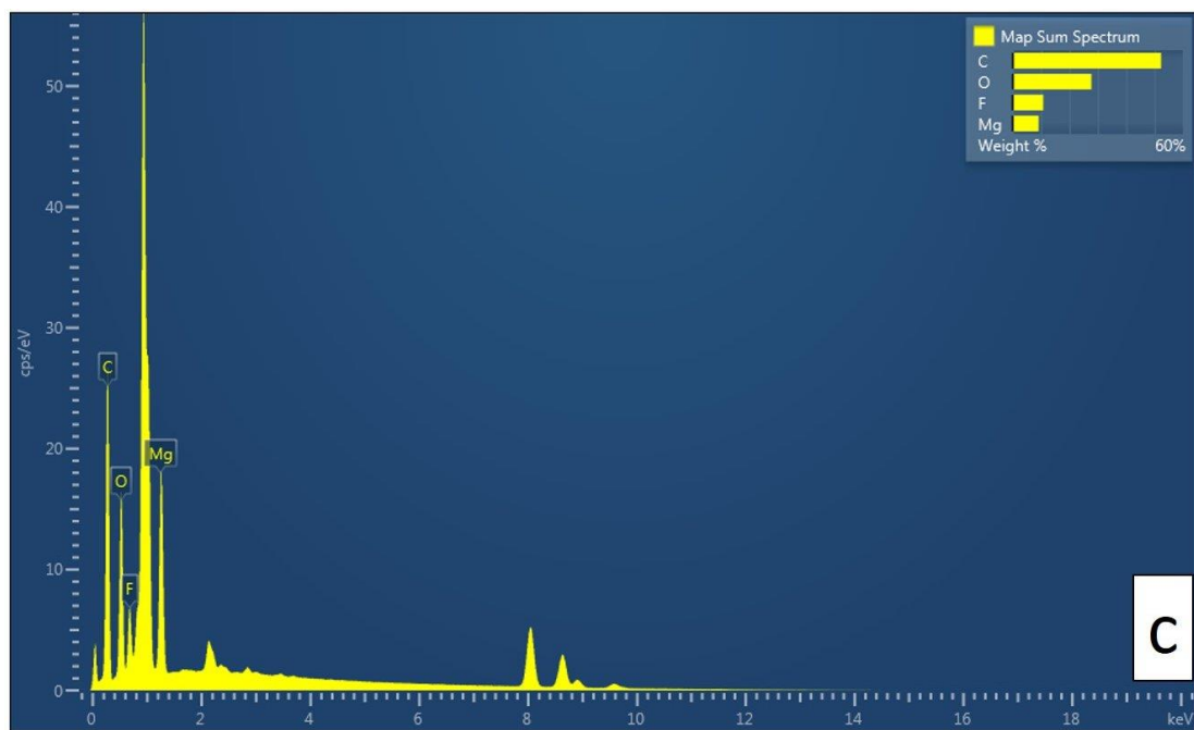
Figure 4.6. (a) EDS regional, (b) EDS mapping, and (c) EDS spectra analysis results of nanosized MgBDC MOF particles
