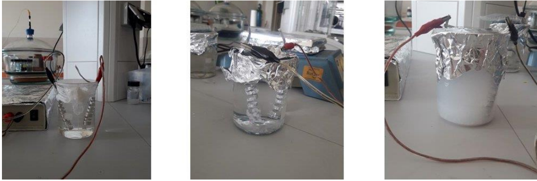
Figure 3.2. Experimental setup of nanosized MgBDC MOF synthesis via the electrochemical method
