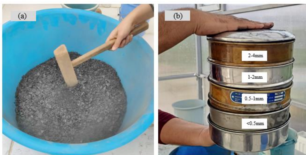
Figure 3.1. (a) Manual crushing of biochar (b) sieving biochar through different mesh sizes for separation
