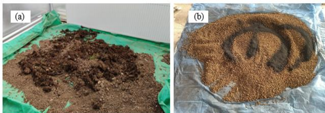
Figure 3.2. (a) Experimental soil kept for air drying, (b) Application of biochar with air-dried and sieved soil.
