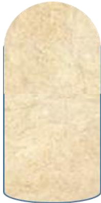
Figure 2.12. Final form of rigid polyurethane foam produced in PET bottle.
