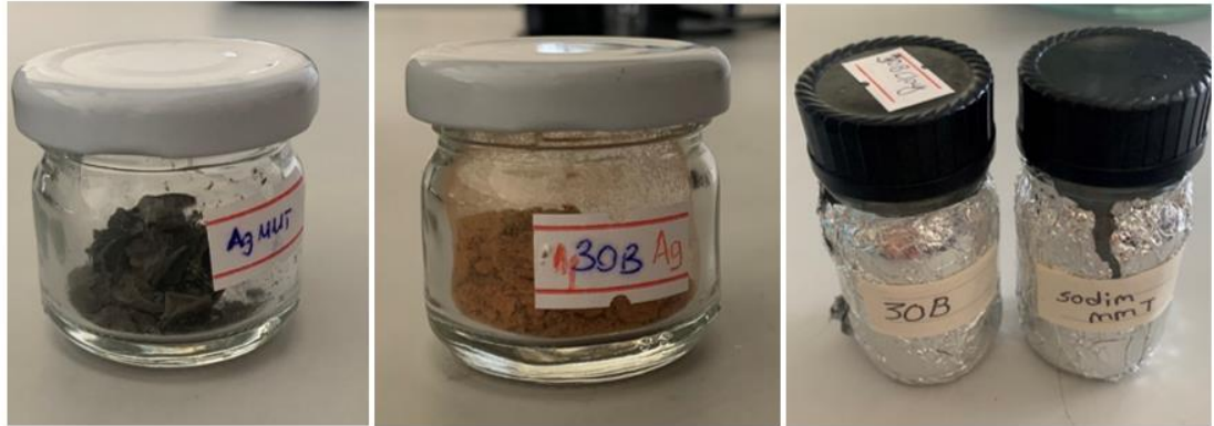
Figure 2.6. Modified nanoclay Ag MMT, Ag 30B and unmodified nanoclay Na MMT, 30B.
