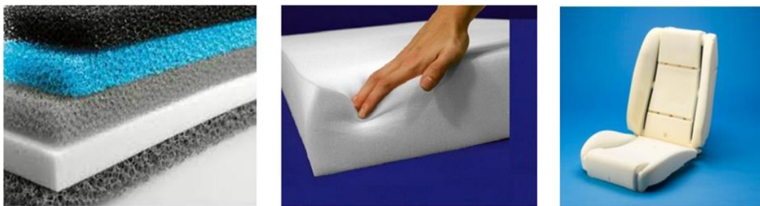
Figure 1.4. Flexible polyurethane foam applications are used in our daily life (Anonymous, 2021a).
