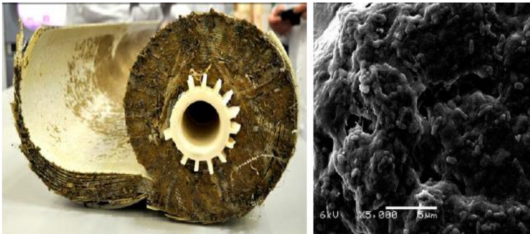
Figure 2.11. Occurrence of bio fouling by microorganism in RO membrane (
