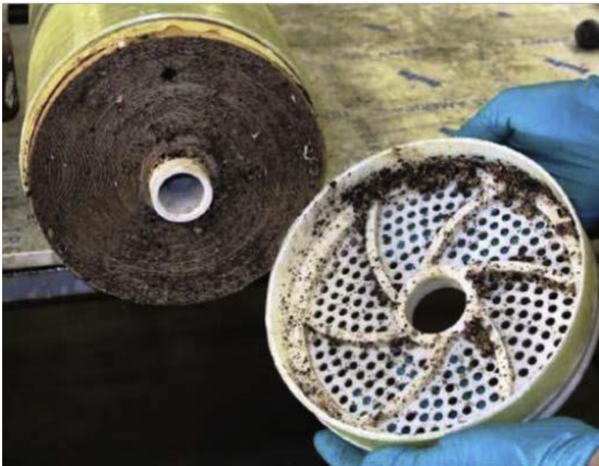
Figure 2.12. Shows the sample of particulate fouling due to suspended solids (Voutchkov, 2017).
