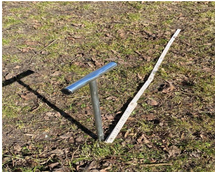
Figure 3.3. Collection of soil material using special sampler
