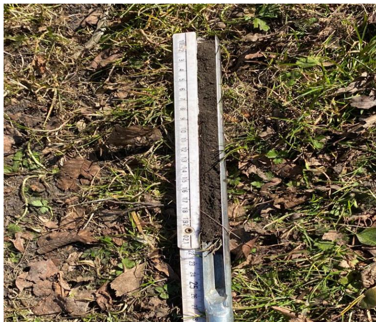
Figure 3.4. Soil samples collection at 0-20 cm depth
