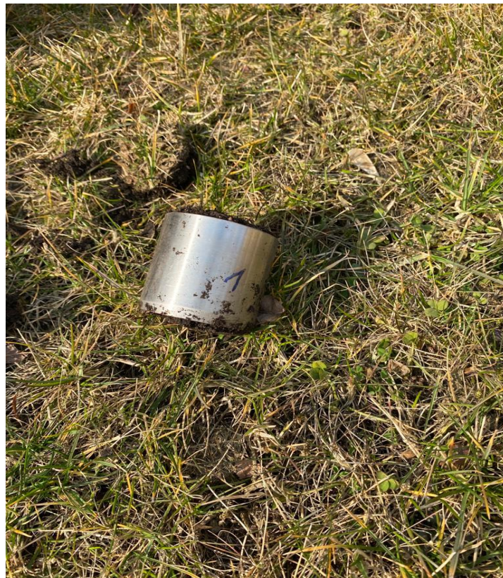
Figure 3.6. Undistributed soil sample in metal cylinder
