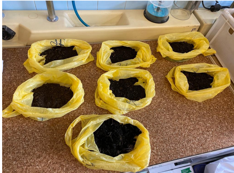
Figure 3.5. Drying of collected soil samples at room temperature
