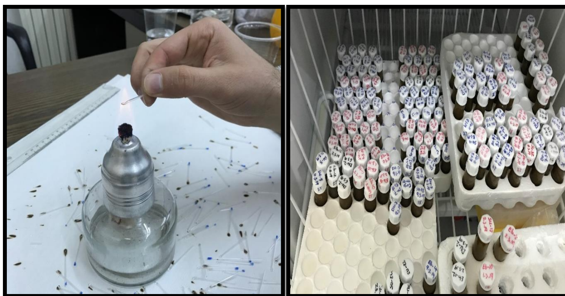
Figure 3.10. (A), Preparation of micro-haematocrit glass tube by using gas burner. (B), tubes inside refrigerator containing micro-haematocrit glass tube
