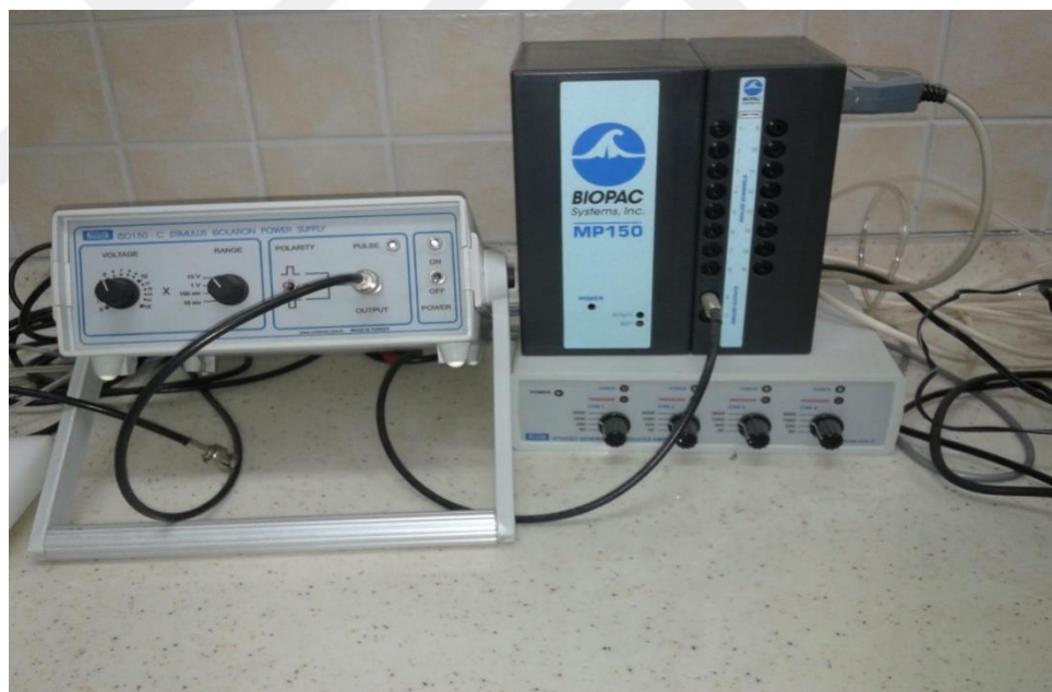
Figure 2.3. Photo of data acquisition system and transducer amplifier
