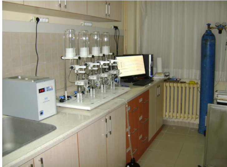
Figure 2.1. Photo of the isolated tissue bath system
