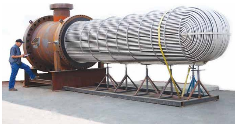
Figure 2.15. Tube bundles of Shell and tube heat exchanger (Anonymous.9, 2019)
