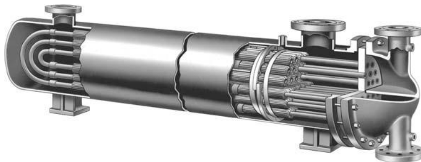
Figure 2.17. Finned U-tube (Thakore and Bhatt, 2007)
