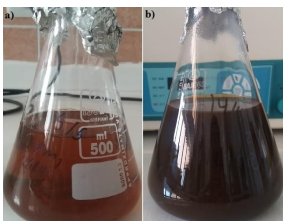
Figure 3.2. Synthesis of silver nanoparticles by strain CPM1 culture broth. (a) culture broth and silver nitrate solution, (b) culture broth and silver nitrate solution after 7 days
