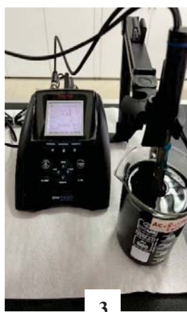
Figure 3.6. Showing of (1) Stainless steel horizontal reactor, (2) 425 µm sieve, (3) pH meter, (4) electronic balance.
